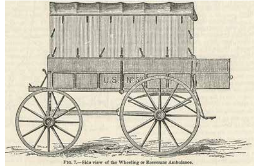
Side view of the Rosenkrans or Wheeling ambulance carriage design.
